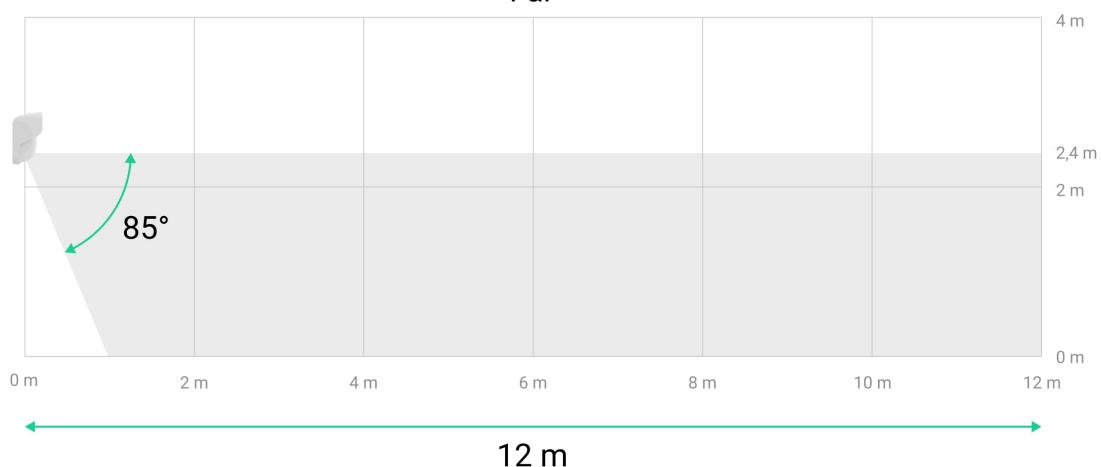
When choosing the installation site, consider the detector's horizontal viewing angle and the width of the detection zone. Incorrect placement of the detector may cause false alarms.
