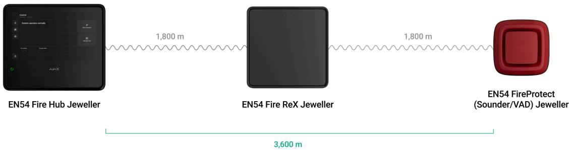
The communication range between EN54 Fire ReX Jeweller and the connected device is limited by the device's radio signal range. It is provided in the device's technical specifications available on the website and in the user manual.
