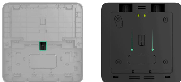
**4.** Prepare the holes for routing cables in advance. Drill the holes in the bottom, side, or top of the enclosure, or break off the perforated part on the back panel.
