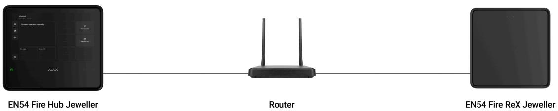
EN54 Fire ReX Jeweller supports connection to the CIE via radio protocols and Ethernet. With the cable connection, a single Ajax system can cover sites such as an office center with underground parking, a metal hangar, or a warehouse complex consisting of several large buildings. Ethernet can be the only communication channel or work in parallel with Jeweller and Wings. If EN54 Fire ReX Jeweller connects to the CIE via both Ethernet and radio communication channels, Ethernet is prioritized.
