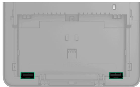
**3.** Remove the SmartBracket mounting panel. To do this, press the button and slide the mounting panel down.
