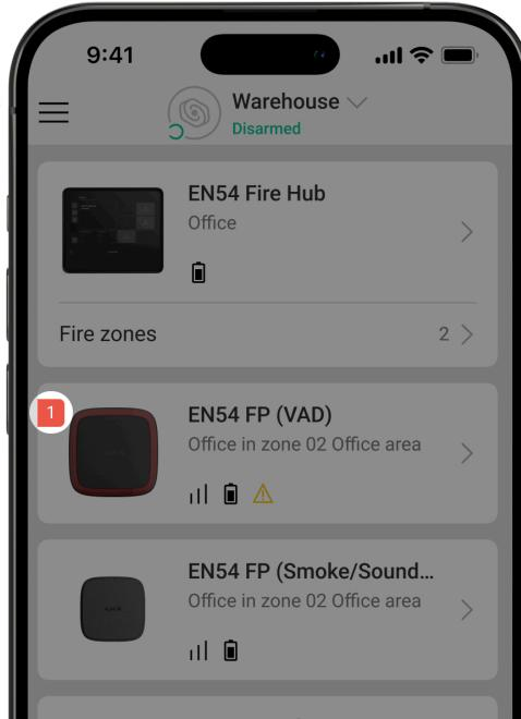
When an EN54 FireProtect (VAD) Jeweller fault is detected, an Ajax app displays a fault counter on the device icon. All faults are indicated in the device states. Fields with faults are highlighted in yellow. Also, faults are displayed in the **Control** tab of the CIE display. More details about the fault can be found in the **Event center** or **Fire zones** tabs of the CIE.
