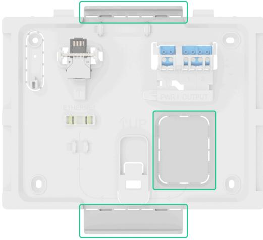
3. Run the power, Ethernet, and optionally signal cables into the CIE enclosure.
