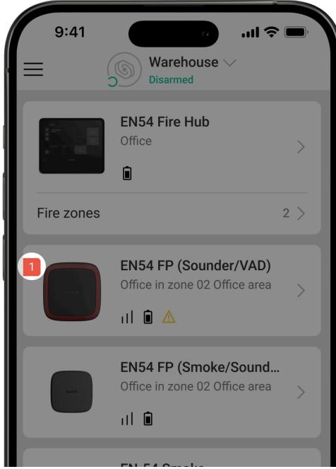
When an EN54 FireProtect (Sounder/VAD) Jeweller fault is detected, an Ajax app displays a fault counter on the device icon. All faults are indicated in the device states. Fields with faults are highlighted in yellow. Also, faults are displayed in the **Control** tab of the CIE display. More details about the fault can be found in the **Event center** or **Fire zones** tabs of the CIE.
