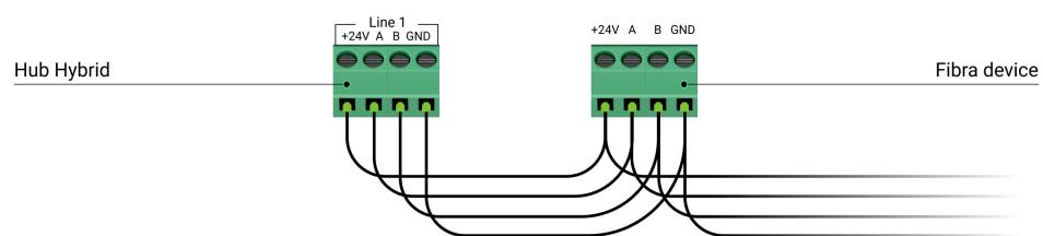
2. If Superior KeyPad Outdoor Fibra is the last device on the line and you are using the **Beam (Radial) connection**, install a terminating resistor on the two contacts by connecting it to the signal terminals of the device. Terminating resistor (120 Ohm) is included in the hub complete set. When the **Ring connection** is used, a terminating resistor is not needed.
