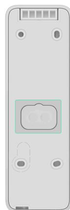
**5.** Run the cable from the hub into the keypad enclosure through the hole that was made.
