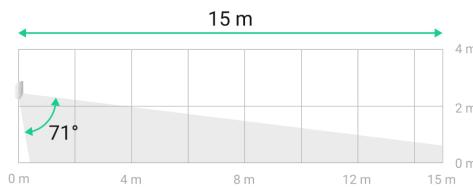
Vertical characteristics of the motion detection area
