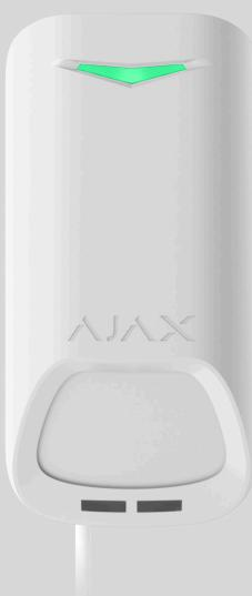
**Superior MotionProtect Plus G3 Fibra** is a wired motion detector. It detects movement at a distance of up to 15 meters. In addition to using the IR sensor, the detector applies an additional radio frequency scan with a K-band microwave sensor that filters out infrared interference. Also, it features an anti-masking system that detects attempts to block the detector's field of view. The device is designed for indoor use only and complies with EN 50131 (Grade 3) requirements.
