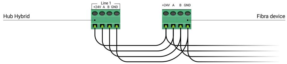
2. If Superior MotionProtect Plus G3 Fibra is the last device on the line and you are using the **Beam (Radial) connection**, install a terminating resistor on the two contacts by connecting it to the signal terminals of the device. Terminating resistor (120 Ohm) is included in the hub complete set. When the **Ring connection** is used, a terminating resistor is not needed.
