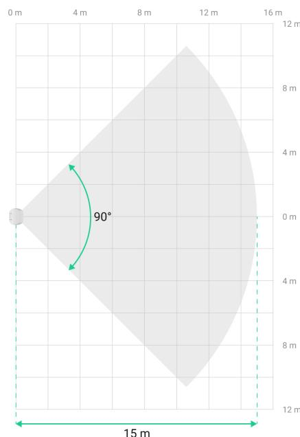
Horizontal characteristics of the motion detection area
