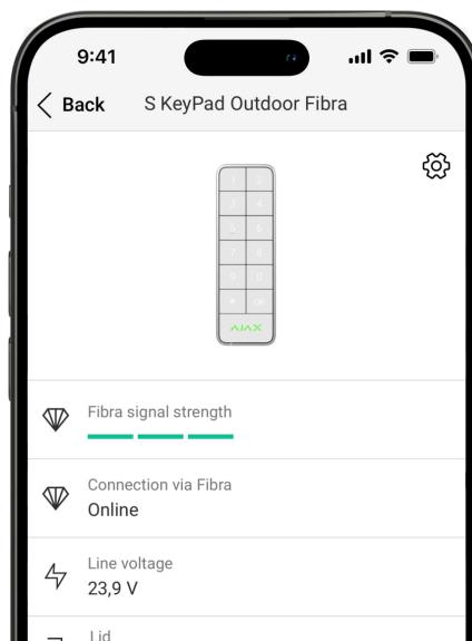
The states include information about the device and its operating parameters. The states of Superior KeyPad Outdoor Fibra can be found in Ajax apps:
