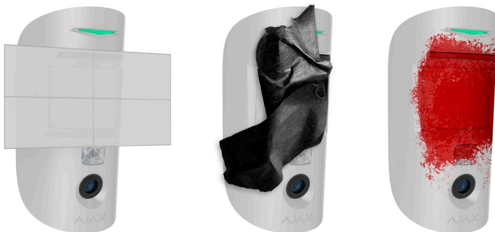
**Masking** is an attempt to block the view of the detector by painting over it, covering it, placing an obstacle in front of the detector lens, or otherwise.
