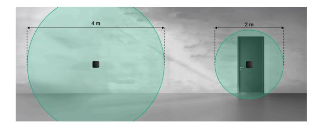
Joints or irregularities in the design of the protected surfaces can impair signal transmission. For example, doors with hinges should have a dedicated detector to ensure proper coverage.
