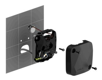
After completing all these installation steps, you can add the device to the hub.
