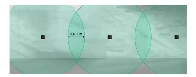
It is recommended that detectors be installed on each plane (walls, floor, ceiling) of the protected premises. If a single device cannot achieve the required coverage radius, several devices should cover the area so that their detection radii overlap by 0.5–1 m.
