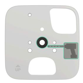
**1. Drill the anchor hole**. Use a drill to create a hole in the concrete surface with a diameter of 10 mm and a depth of at least 60 mm.
