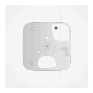
9. Remove the Superior SeismoProtect G3 Fibra lid and drill holes for the cable. When using the bundled armored cable, carefully break out the perforated part to bring the cable out. When using other cables with smaller diameters, drill holes for the cable at low speeds.
