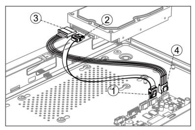
**Figure 1-11 Connect Cables**
