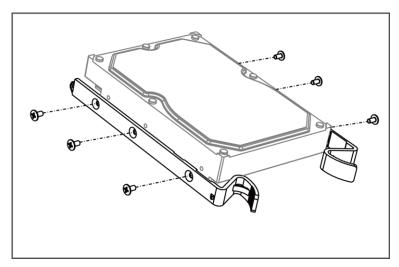
Figure 1-5 Fix Mounting Ears to HDD
