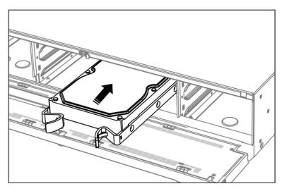
Figure 1-7 Insert HDD
