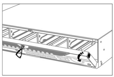
Figure 1-6 Open Front Panel
