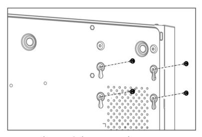
Figure 1-12 Fix HDD to Device Bottom
