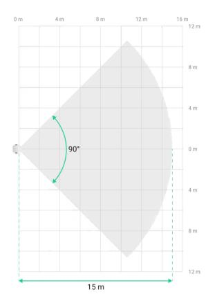
The direction of the detector sensors should be perpendicular to an alleged intrusion path into the facility.
