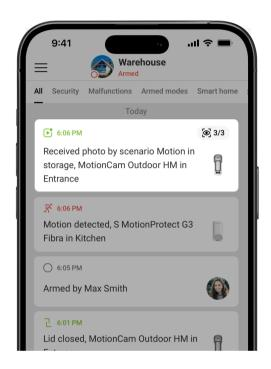
The **Photo by scenario** feature allows you to create a scenario for motion detectors supporting photo verification. These detectors will take pictures in case of alarms from specified Ajax devices.
