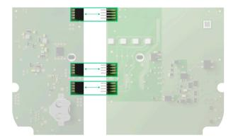
**9.** Install or remove the jumper, depending on the operating mode.
