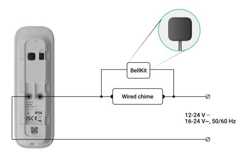
Once DoorBell and BellKit are connected to a wired chime, you need to configure the chime connection in an Ajax app. Before configuring, ensure that DoorBell is added to the system.
