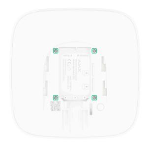
**5.** Remove the screws attaching the boards to the device body.
