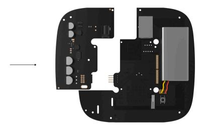
Please note: the board contacts should be plugged in the bottom row of the connector (closest to the board). When connected correctly, the boards are on the same level.
