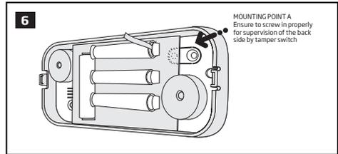
3. When installing EWS3, follow the recommendations for the installation to achieve the strongest wireless signal:
