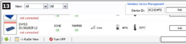
8. Upon the successful pairing process, the message indicated next to EWS3 device icon will turn to **CONNECTED**. If the attempt to pair is unsuccessful, try to move EWS3 closer to the ELDES alarm system and pair anew.
