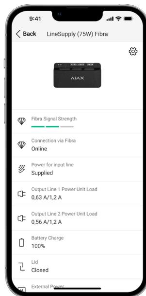
The states include information about the device and its operating parameters. You can find the states of LineSupply in the Ajax app:
