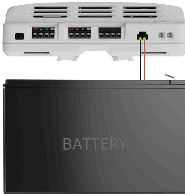
**10.** Connect the main power supply to the appropriate module connector.
