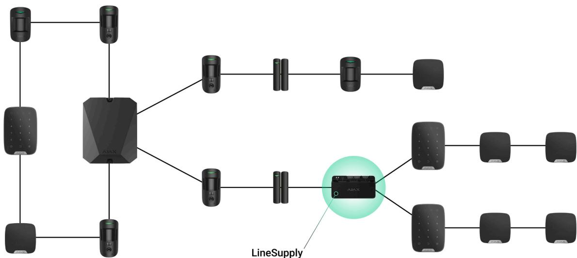
While Ajax systems support **Beam** and **Ring** topologies, avoid connecting the module's Fibras output lines in a **Ring** topology.
