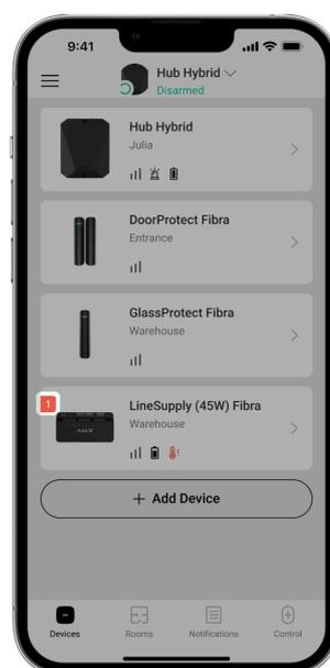
When a LineSupply malfunction is detected, the Ajax app displays a malfunction counter on the device icon. All malfunctions are indicated in the module states. Fields with malfunctions will be highlighted in red.
