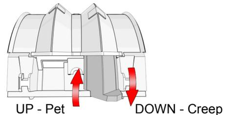
Remove detector assembly as described in Step 1. When selector is UP, Pet Mode; when DOWN, Creep Zone is active and there is no Pet Immunity. Above 2.4m Pet Immune should be OFF (lever down Pet OFF), see installation height note\*.
