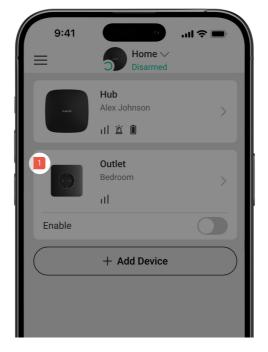
When Outlet [type F] malfunction is detected, the Ajax app displays a malfunction counter on the device icon. All malfunctions are indicated in the outlet's states. Fields with malfunctions will be highlighted in red.
