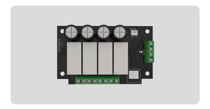
**MultiRelay Fibra** is a module to control electrical appliances' power supply remotely. The device has four relays with electrically isolated dry contacts. The relays can control the power supply of electrical appliances connected to the circuit. To change the states of the relays, use the **Ajax apps**, create **automation scenarios**, or press **Button**.
