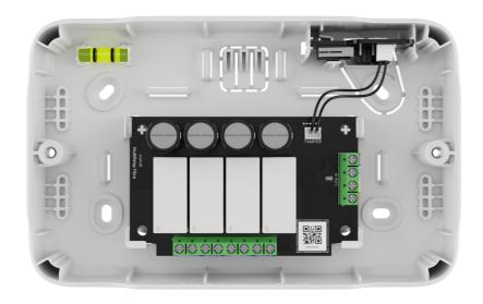
We recommend installing MultiRelay into Case. The casing is sold separately and available in multiple versions. Installing a single module, several modules, or several other devices into Case is possible.
