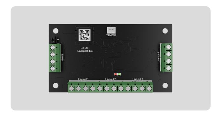
**LineSplit Fibra** is a module designed to split one Fibra line into four ones. Each device output line can have a length of up to 2,000 meters when connected using the U/UTP cat.5 twisted pair cable. LineSplit can be installed at any point of the line, in particular after another LineSplit.
