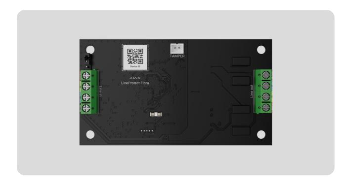
**LineProtect Fibra** is a module designed to protect devices on the Fibra line from short circuit and sabotage: 110/230 V~ voltage supply to the line, hit with the stun gun.
