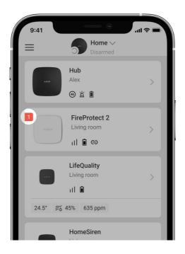
If FireProtect 2 malfunction is detected (for example, there is no connection with the hub), the malfunction counter is displayed in the device field in the Ajax apps.
