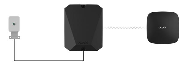
MultiTransmitter can be used to connect alarm and auxiliary request buttons, indoor and outdoor motion detectors, as well as detectors that track opening, vibration, glass breaking, fire, gas and water leakage, etc.
