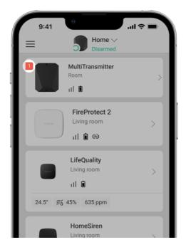
If the MultiTransmitter malfunction is detected (e. g., loss of connection with the hub via Jeweller), the Ajax app displays a malfunction counter in the upper left corner of the device icon.
