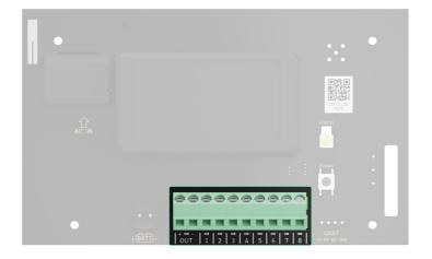
• BATT – input for the 12 V- backup power connection.
