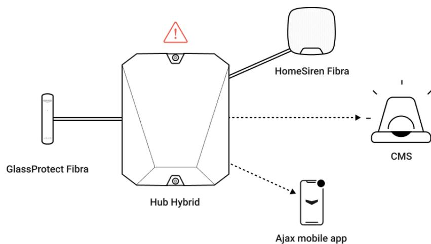
**GlassProtect Fibra** is a wired glass break detector. It responds to glass breaking using a built-in electret microphone. The detector's microphone using the DualTone digital algorithm only responds to sound vibrations characteristic of the sound of glass breaking, cutting off false alarms.
