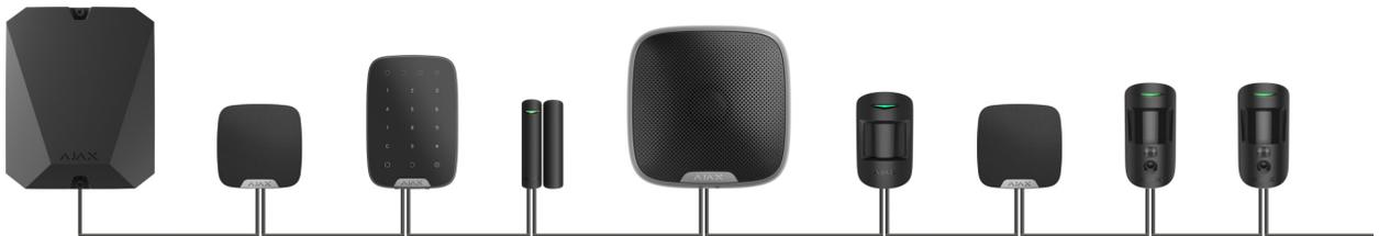
**Ring connection** occupies two bus outputs of the hub. If the ring breaks in one place, no device will be deactivated. The ring reconfigures into two lines, which continue to operate normally. Users and the security company will receive notification about the break.
