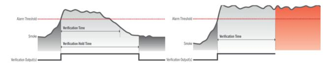
Signal cleared before Verification Time expires – no signal. Without Verification Hold Time the panel would return to normal as soon as the signal dropped below alarm threshold.
