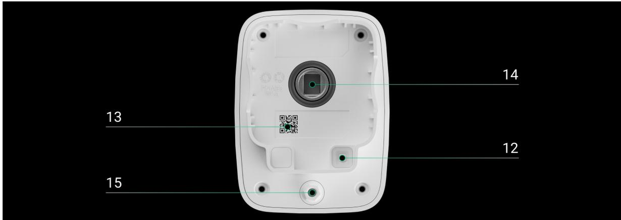
12. Tamper button. Reacts to the removal of the electric actuator from the mount.
