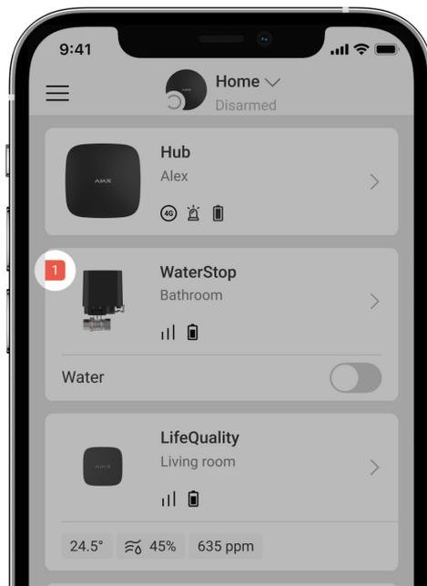
If a malfunction is detected in WaterStop (for example, there is no connection with the hub or range extender), the malfunction counter is displayed in the device field in Ajax app.
