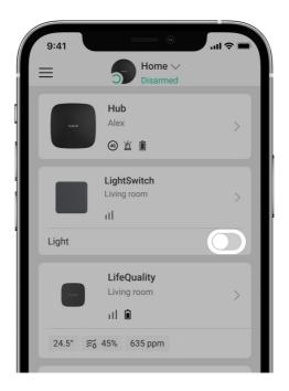
Press the switch in the **LightSwitch** field in the **Devices** menu in the Ajax app, and the state of the switch contacts will change to the opposite; lighting will be switched off or on. This way, system users can remotely control the lighting. For example, switch on the light in the room in advance before entering the room.
