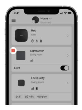
When a device identifies a fault (for example, there is no connection with the hub), the Ajax app displays a fault counter in the device field.
