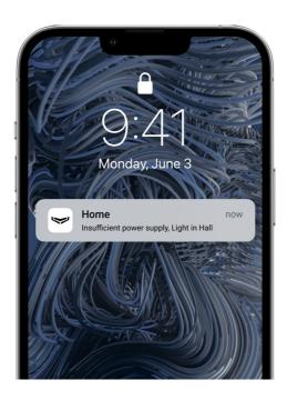
LightSwitch regularly measures the switching current. If LightSwitch controls the power of a lighting device with insufficient power (up to 5 W), the system will notify the users of the Ajax system. In this case, it is necessary to replace the lighting device with a similar one with higher capacity or to connect a bundled capacitor in parallel with the lighting device.
