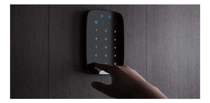
You can activate the keypad by swiping your hand over the touch panel from top to bottom. When activated, the backlight on the keypad will turn on and a beep will sound (if enabled).
