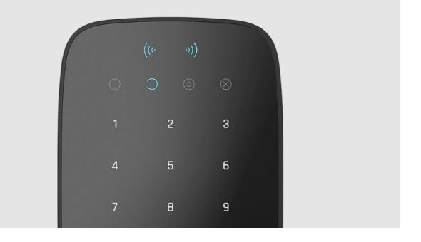
You can use the KeyPad Plus without ambient lighting as the keypad has a backlight. The pressing of the buttons is accompanied by a sound signal. The backlight brightness and keypad volume are adjustable in the settings. If you do not touch the keypad for 4 seconds, KeyPad Plus reduces the backlight brightness, and 8 seconds later goes into power-saving mode and turns off the display.
