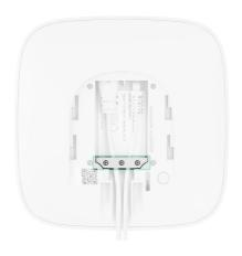
**4.** Slide ReX 2 onto the mounting panel. After installation, check the tamper status in the Ajax app and then the quality of the panel fixation. You will receive a notification if an attempt is made to tear the range extender off the surface or remove it from the mounting panel.
