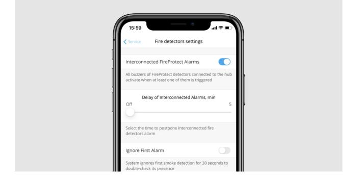
5. If necessary, activate the **Ignore First Alarm** option. This setting is recommended for premises with potential sources of false alarms. For example, if the device is installed in a place where dust or steam can get into the detector.
