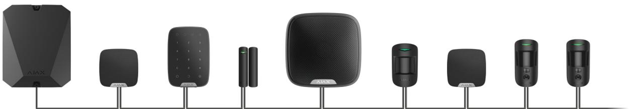
**Ring connection** occupies two line outputs of the hub. If the ring breaks in one place, no device will be disabled. The ring reconfigures into two lines, which continue to operate normally. Users and the security company will receive notification of the break.
