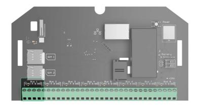
Hub Hybrid (2G) / (4G) has 8 buses. Numbers from 1 to 8 are indicated on the control panel board.
