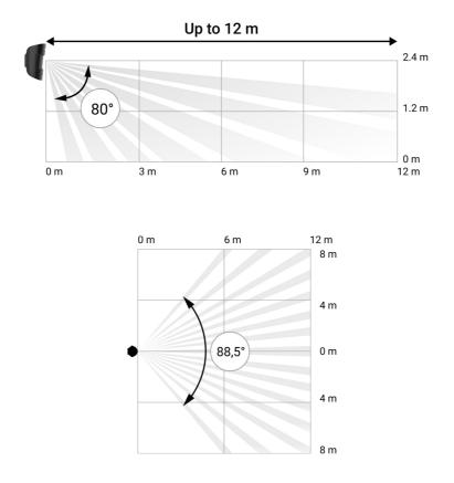
We recommend installing the detector at the height of 2.4 meters.
