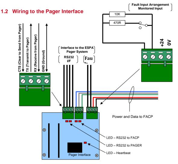
The Serial Interface follows the standard RS232 interface connections. Run the cabling in rigid conduit or use fire rated cable. Note: Maximum distance of 3m (10ft) between the Interface and the Pager.
