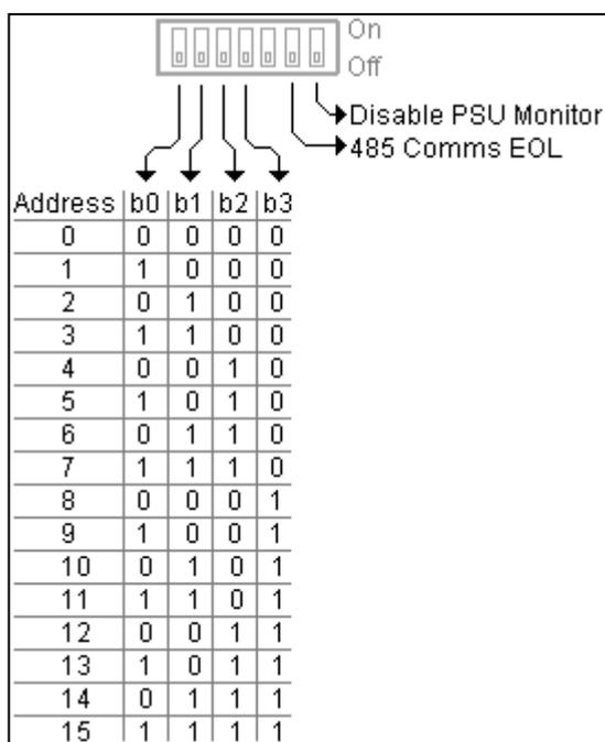
Each card connected to the 485 Communication Line (PBUS) must have its own address. This address should be set so that it matches the corresponding card within the Advanced PC Config Tool design.
