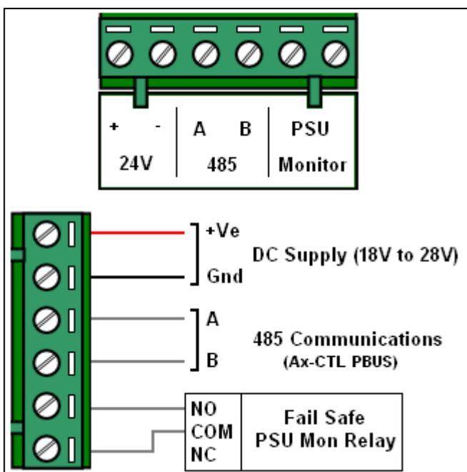
The Terminal block provides the main contact point between a card, or set of daisy chained cards, and the parent FACP.
