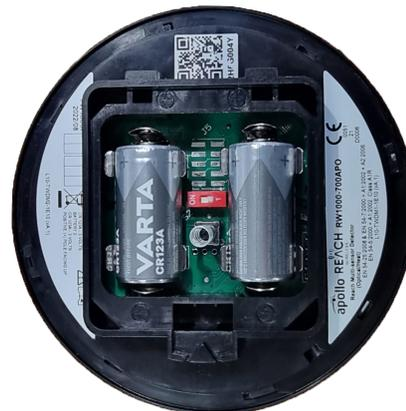
Once the device has been prepared, follow the on-screen instructions and set the device switch to the '1' position.
