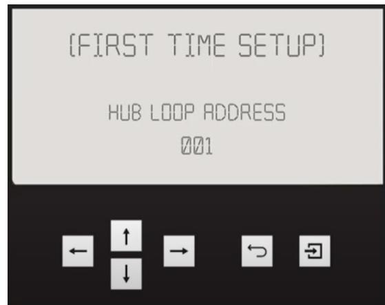
Once first-time setup is complete, the Hub will navigate you to the **CONFIGURATION MODE** menu.
