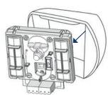
Remove the sounder interface module from the base.
