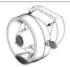
Remove the mounting from the sounder by pulling apart the two pieces.
