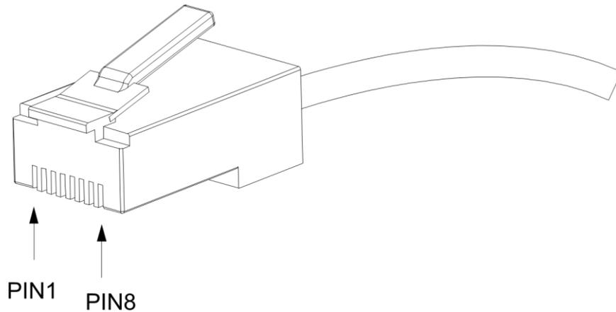
Figure 3-6 RJ-45 connector of the console port
