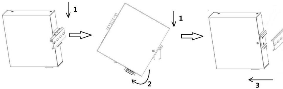
Figure 3-2 track installation diagram
