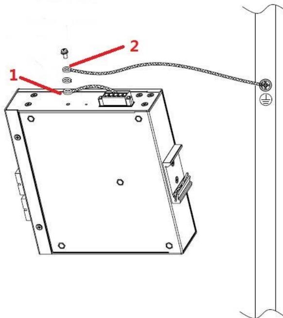
Figure 3-3 track Equipment grounding
