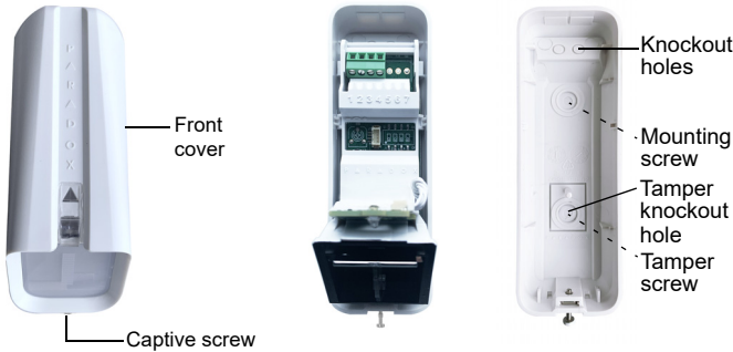
Figure 1 – Removing the Front Cover
