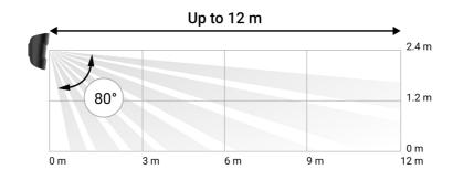
We recommend installing the detector at the height of 2.4 meters.
