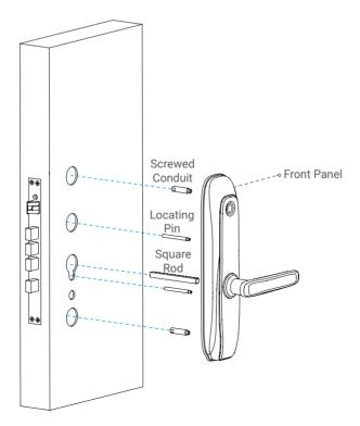
3 Fix the fixed plate and rubber pad into the door with ① locating pin and ② tighten sleeve.
