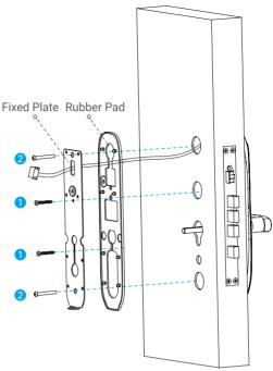
4 With the secure knob keeping upright, fix the rear panel with screws as shown below.
