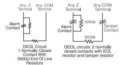
**NOTE:** Only normally closed detection devices can be used with this type of zone supervision. Only one normally closed contact can be connected to each zone; multiple detection devices/ ontacts on one loop are not allowed, the tamper condition will not be monitored.
