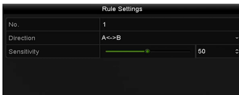
Figure 8-13 Set Line Crossing Detection Rules
