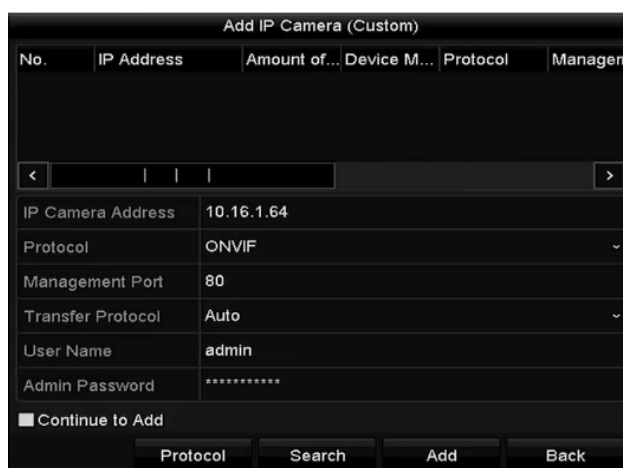
Figure 2-25 Custom Adding IP Camera Interface
