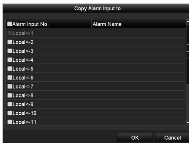
Figure 8-8 Copy Settings of Alarm Input
