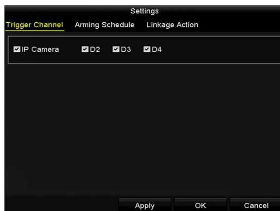
Figure 5-17 Set Trigger Camera of VCA Alarm
