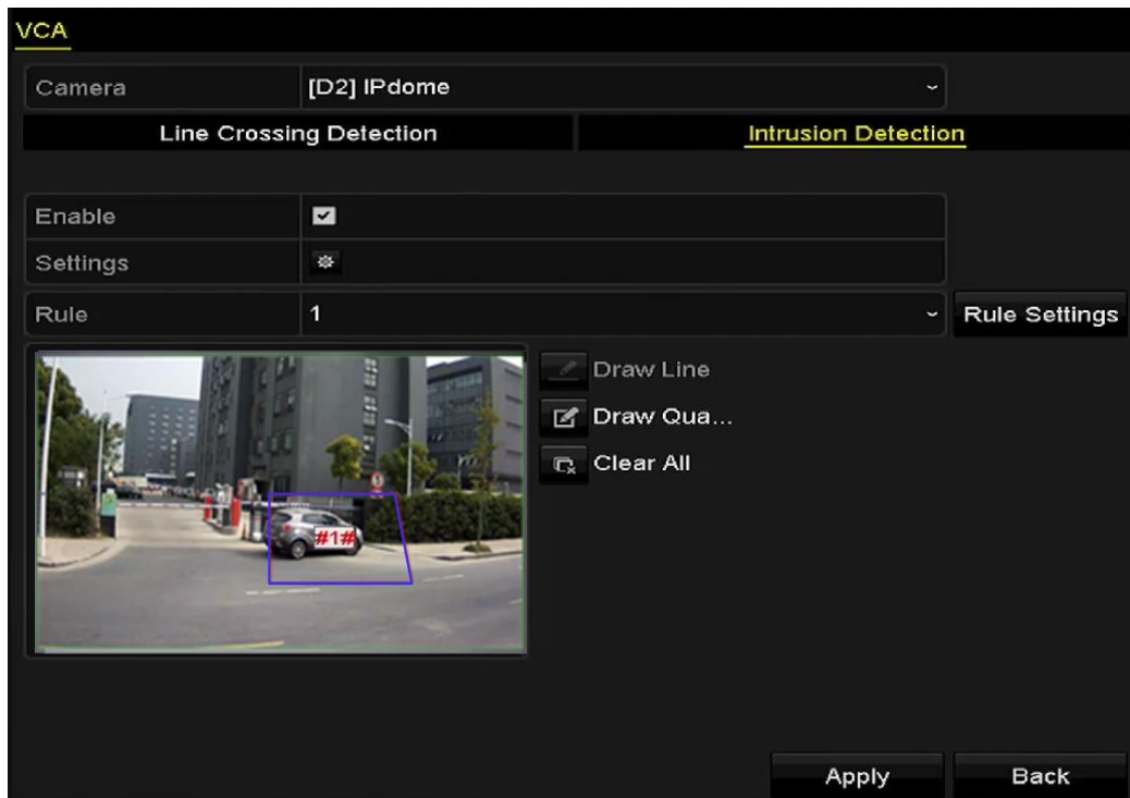
Figure 8-16 Draw Area for Intrusion Detection
