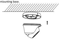
Figure 2-4 Secure the Camera with Mounting Base
