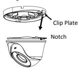
Figure 2-6 Disassemble the Camera
