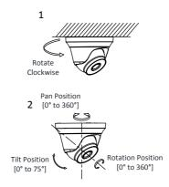
Figure 2-15 3-axis Adjustment
