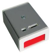
To reset, a specific key included in the package is necessary. 4-terminal connection: 2 for contact and 2 for anti-tampering. Version 484-ME: LED memory with central reset (by cutting power supply), button with spring return.
